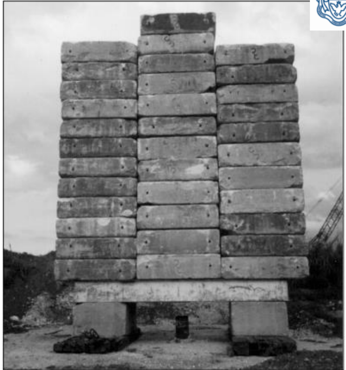
Figure 9-67. Typical compression load test arrangement using a weighted platform (FHWA, 2006a).
