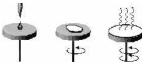
Fig. 26. Stages of the spin coating process: deposition of the sol, spin up, spin off and gelation by solvent evaporation.
