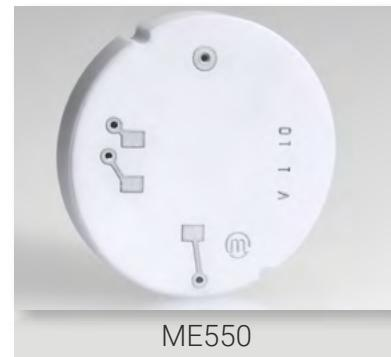
Put simply, ceramic pressure sensors operate at their calibrated values longer than other conventional models. Plus, ceramic is inherently resistant to corrosion and abrasion from particles, making these sensors compatible with most process media. Ceramic types can also withstand higher operating temperatures and pressures but are sensitive enough to measure low pressures while tolerating high overpressures.
