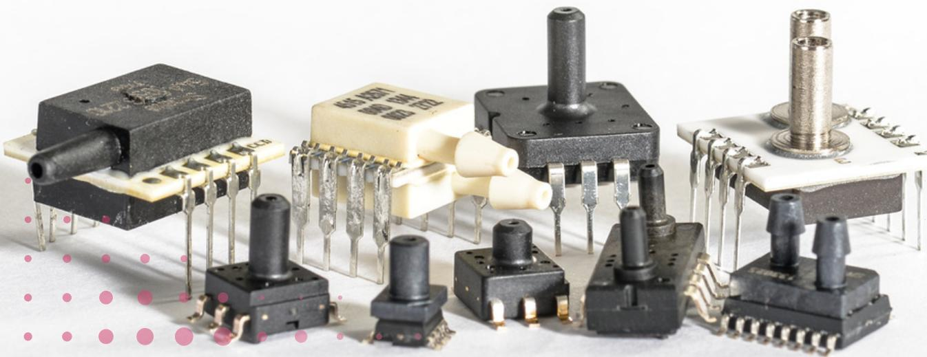
The advent of microelectromechanical systems (MEMS) technology has resulted in a wide range of pressure sensor style and performance options, allowing for use in an equally wide range of applications, including industrial instrumentation, medical monitoring, HVAC equipment, consumer devices, and many others.
