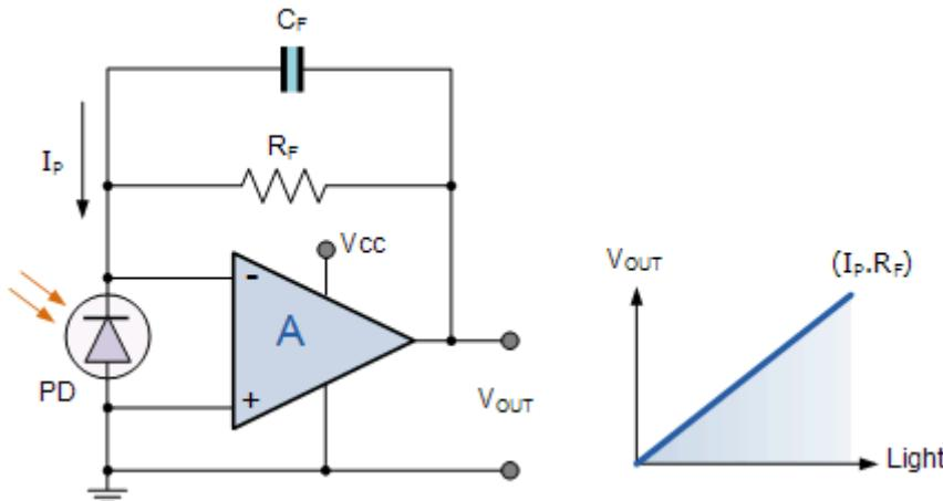
**Photodiodes** are very versatile light sensors that can turn its current flow both “ON” and “OFF” in nanoseconds and are commonly used in cameras, light meters, CD and DVD-ROM drives, TV remote controls, scanners, fax machines and copiers etc., and when integrated into operational amplifier circuits as infrared spectrum detectors for fiber optic communications, burglar alarm motion detection circuits and numerous imaging, laser scanning and positioning systems etc.
