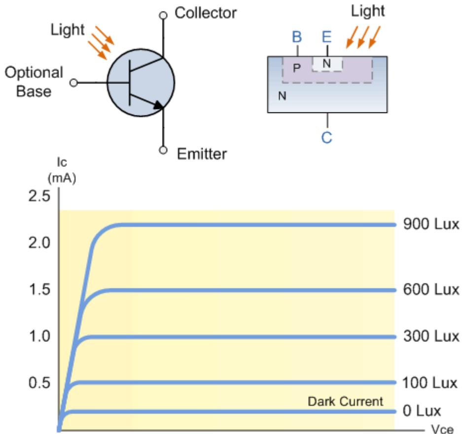
In the NPN transistor the collector is biased positively with respect to the emitter so that the base/collector junction is reverse biased. therefore, with no light on the junction normal leakage or dark current flows which is very small. When light falls on the base more electron/hole pairs are formed in this region and the current produced by this action is amplified by the transistor.
