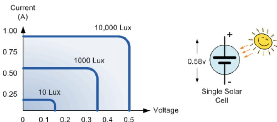
The amount of available current from a solar cell depends upon the light intensity, the size of the cell and its efficiency which is generally very low at around 15 to 20%. To increase the overall efficiency of the cell commercially available solar cells use polycrystalline silicon or amorphous silicon, which have no crystalline structure, and can generate currents of between 20 to 40mA per  $\text{cm}^2$ .
