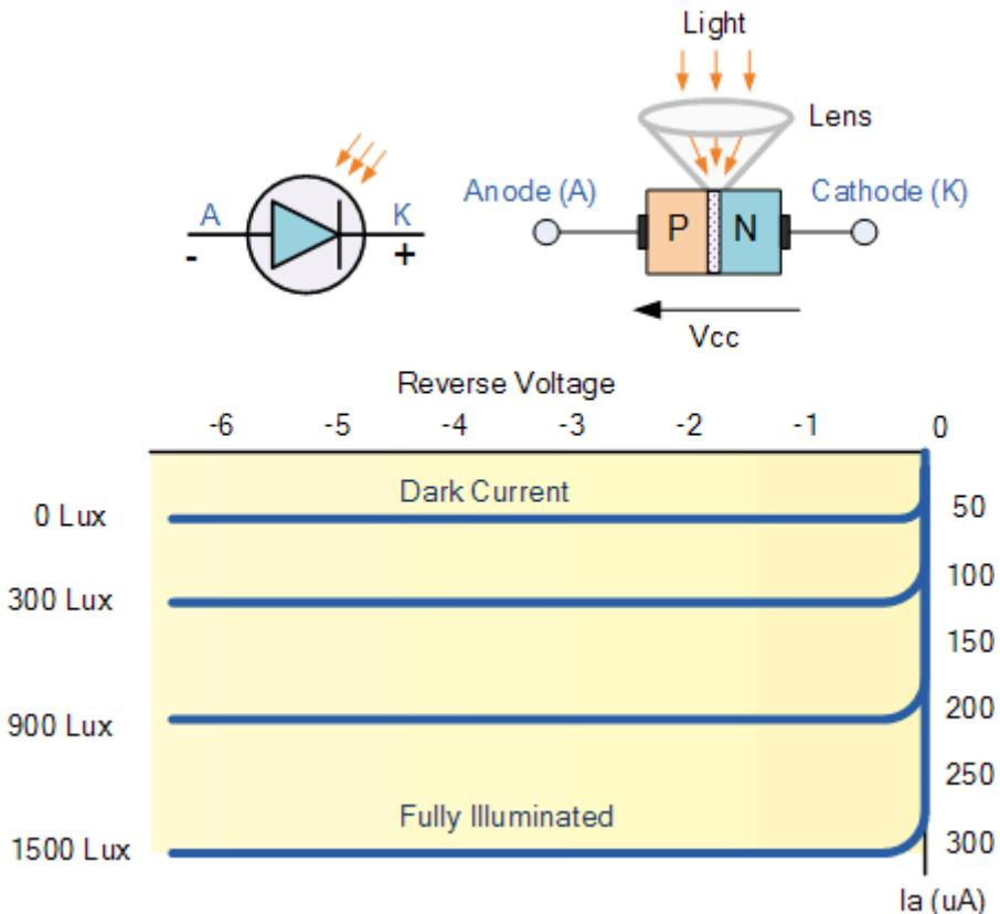
When used as a light sensor, a photodiode dark current (0 lux) is about 10uA for geranium and 1uA for silicon type diodes. When light falls upon the junction more hole/electron pairs are formed and the leakage current increases. This leakage current increases as the illumination of the junction increases.
