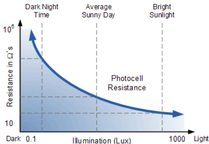
The most used photoresistive light sensor is the **ORP12** Cadmium Sulphide photoconductive cell. This light dependent resistor has a spectral response of about 610nm in the yellow to orange region of light. The resistance of the cell when unilluminated (dark resistance) is very high at about  $10M\Omega$ 's which falls to about  $100\Omega$ 's when fully illuminated (lit resistance).
