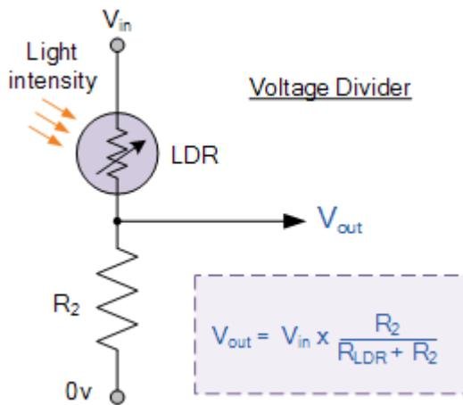
Connecting a light dependant resistor in series with a standard resistor like this across a single DC supply voltage has one major advantage, a different voltage will appear at their junction for different levels of light.
