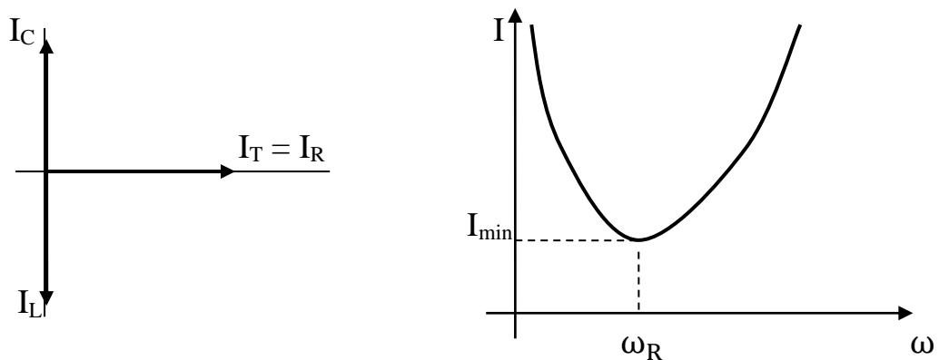
$$\vec{I}_T = \vec{I}_R + \vec{I}_L + \vec{I}_C \quad \therefore \quad I_{\min} = \frac{V_m}{R}$$
