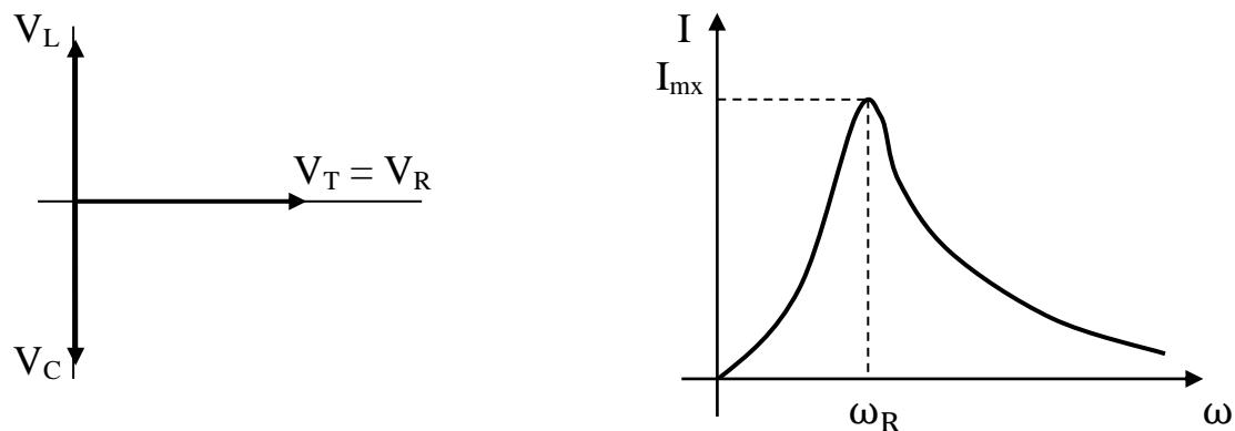
$$\vec{V}_T = \vec{V}_R + \vec{V}_L + \vec{V}_C \quad \therefore \quad I_{mx} = \frac{V_m}{R}$$
