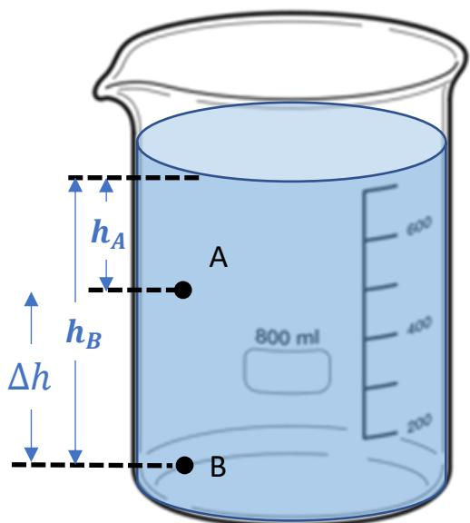
$$\left. \begin{array}{l} p_A = p_{atm} + \delta \cdot h_A \cdot g \\ p_B = p_{atm} + \delta \cdot h_B \cdot g \end{array} \right\} \Delta p = p_B - p_A$$
